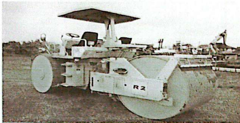
Gambar 8: three wheel roller _ alat pemadat
